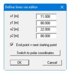
Enter the respective x- and y-coordinates of the start and end point of the line. Activate the "End point = next start point" check box to created a polygon course. After confirming your input the defined line is drawn on the screen. If you go to this menu item a second time the old end coordinates are adopted as start coordinates.
