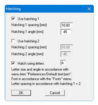
Two different types of hatching are available, for which the line spacing and the angle can be defined. It is also possible to use both simultaneously, if both check boxes are activated.
