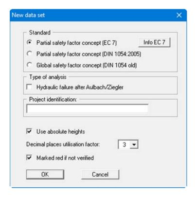
In the first group box the radio buttons are used to specify which safety concept to use for analysis. The hydraulic heave analysis after Aulbach/Ziegler can be activated below this.
