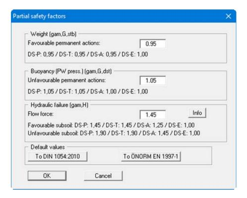
If you press the "Info" button, you will see further information on the subsoil situation (favourable/unfavourable). In the "Default values" group box the partial factors for the various load cases and subsoil conditions given in the DIN 1054:2010 and in the EC 7 can be selected by means of the dialog box reached by clicking the "To DIN 1054:2010" button. The load case designations were altered for the EC 7 partial safety factor concept:
