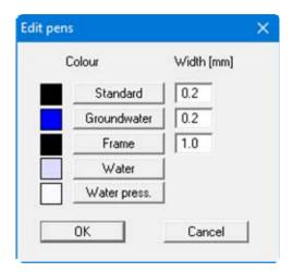
You can edit the pen widths for the elements shown in the dialog box; by clicking on the button with the element designation you can also edit the pen or fill colours.
