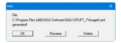
The default location of the file is the folder from which the program is started and, if several files are created, the file is given the file name "Image0.emf" with sequential numbering. If the "Rename" button in the dialog box is clicked, a file selector box opens and the copied area can be saved under a different name in a user-defined folder. Saving can be aborted by pressing the "Delete" button.
