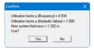
Thus, in order to achieve an optimum utilisation factor, a 1.29 m thick clay liner is required. If you answer "Use?" with "Yes", the system thickness determined here will be used as the new base in "Edit/Soils". The results shown in the legends are automatically adjusted.
