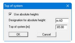
Once you have confirmed your input you will next be presented with a query on how to deal with the existing elevation data for soil strata and groundwater. If you leave the elevations at the same level (= check boxes activated), the originally entered data will not be modified.
