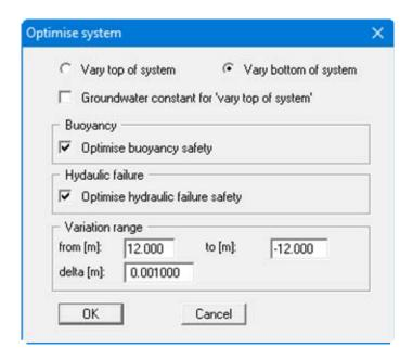
In the upper part of the dialog box you specify whether the top of the system or the bottom is to be varied. If you activate the "Vary top of system" switch, you can additionally specify whether the groundwater level is to be kept constant during variation, or whether it is to be kept at a constant distance to the top of the system.
