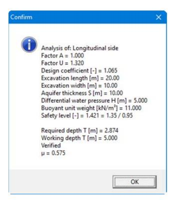
The resulting utilisation factor  $\mu$  is given by division of required T/working T.
