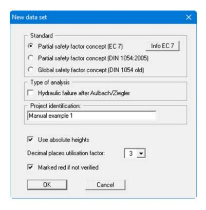
If the "Use absolute heights check box is activated (program default), the height input of soil layers and groundwater will be in absolute coordinates (e.g. in m AD). Otherwise, "Top of system" corresponds to 0.0 m and all height input is positive downwards.
