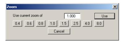
A zoom factor between 0.4 and 8.0 can be entered in the input box. By then clicking on "Use" to exit the box the current factor is accepted. By clicking on the "0.4", "0.6", etc. buttons, the selected factor is used directly and the dialog box closed.
