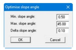
Enter the minimum, maximum and delta for the selected parameter, here the slope angle, and click "**OK**". The optimum value is shown in a message box, in this example the optimum slope angle for a safety factor of 1.41. You can now decide whether to adopt the optimised value in the system parameters. If you do not want to use this value click "**No**".
