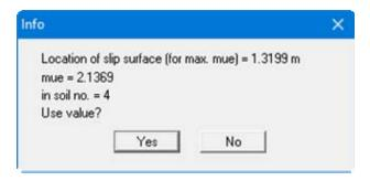
If you click "Yes" the position of the slip surface is adopted in the "System parameters" dialog box (see Section 5.2.3.2) and drawn in the system visualisation at the identified depth.
