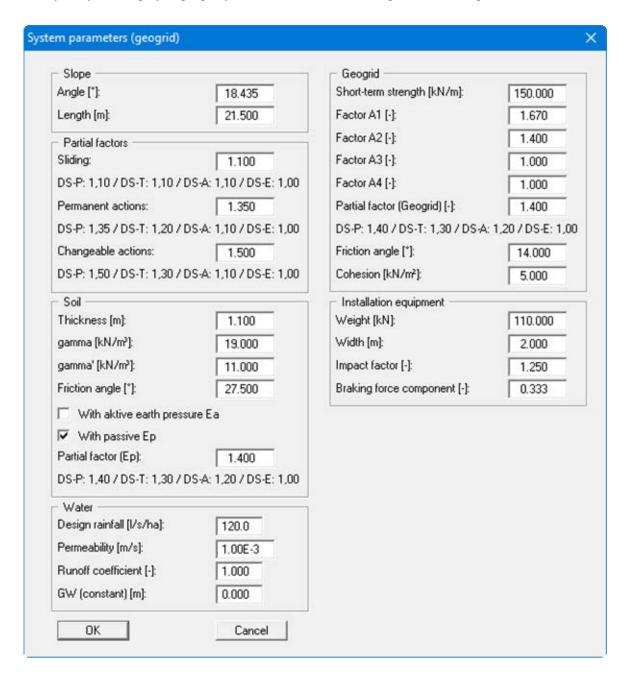
You enter the governing values for the slope, soil, water, geogrids and installation equipment in the respective group boxes. If the *partial safety factor concept* is selected you can also enter the respective partial safety factors in the dialog box.
