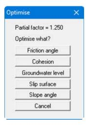
If you are using the *global safety factor concept* you can enter the allowable safety in the dialog box. When using the *partial safety factor concept* the partial safety factor for the shear coefficients as defined in "Edit/System parameters" is displayed.
