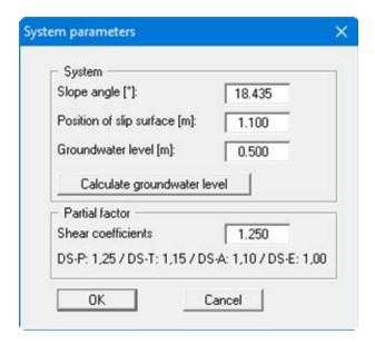
Only the soil properties are defined in the multi-layer system-specific "Edit/Soils" menu item (see Section 5.2.4). If you are using the *partial safety factor concept*, you can also enter the partial safety factor for the shear coefficients in the dialog box.
