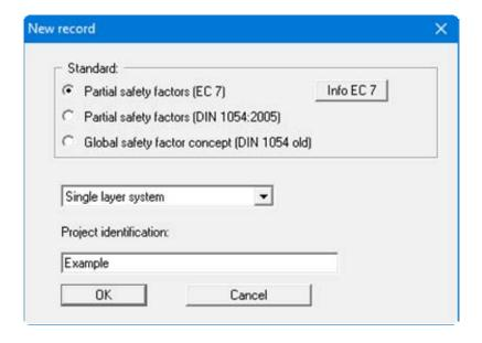
In the upper group box of this dialog box select the safety factor concept for analysing your new system. The type of system can be specified in the middle drop-down list box. Select from the following settings:
