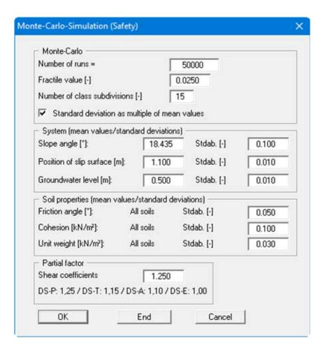
The mean and the standard deviation are given for each parameter. If the check box "**Standard deviation as multiple of mean values**" is activated you will be presented with a percentage standard deviation relative to the mean value of the parameter. Deactivate this check box if a fixed value is to be used in calculations.
