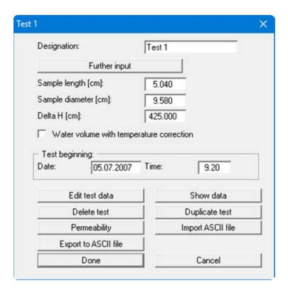
In the input boxes define the sample via length, diameter and delta H. By activating the "Water volume with temperature correction" check box, a temperature correction can be accomplished for test evaluation. Date and time of the test beginning can be entered below.
