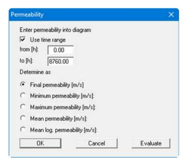
Clicking the "Evaluate" button displays a result box with the corresponding permeability data, as it is also shown in the diagram table.
