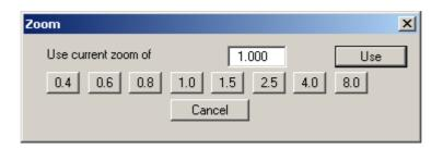
A zoom factor between 0.4 and 8.0 can be entered in the input box. By then clicking on "Use" to exit the box the current factor is accepted. By clicking on the "0.4", "0.6", etc. buttons, the selected factor is used directly and the dialogue box closed.
