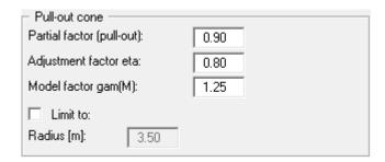
The radius of the pull-out cone may be limited. The allowable heave is specified for determination of R(E,k) of tension piles.
